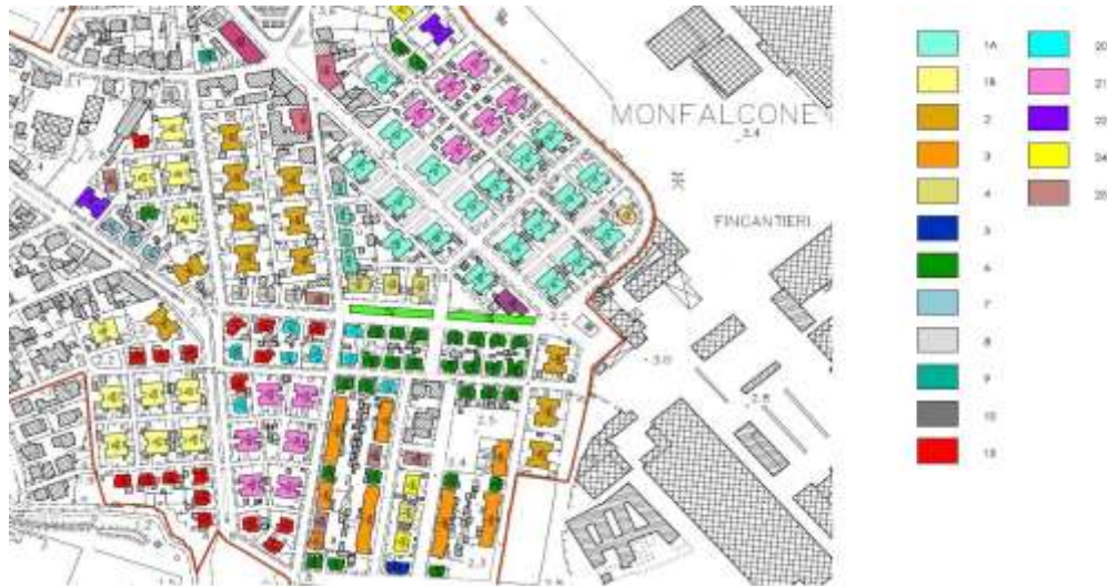
Figure 6. Situation Plan (2010) of the Building Stock Typologies in the Workers' Village: The Continuous Red Line Borders the Perimeter of the Recovery Plan Scope. In the Key Legend, Codes 1A and 1B Refer to Eight-dwelling Houses with Separate Entrance, which Constitute the Focus of this Study Source: Project Group of Panzano Municipality for Panzano Recovery Plan, 2010a.
