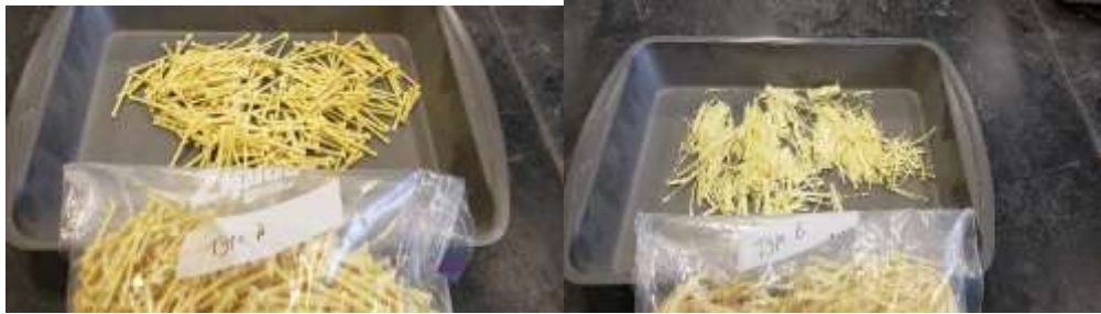
Figure 1. Fibers used for the Study: Aramid fiber Type A (left) and Type B (right)
