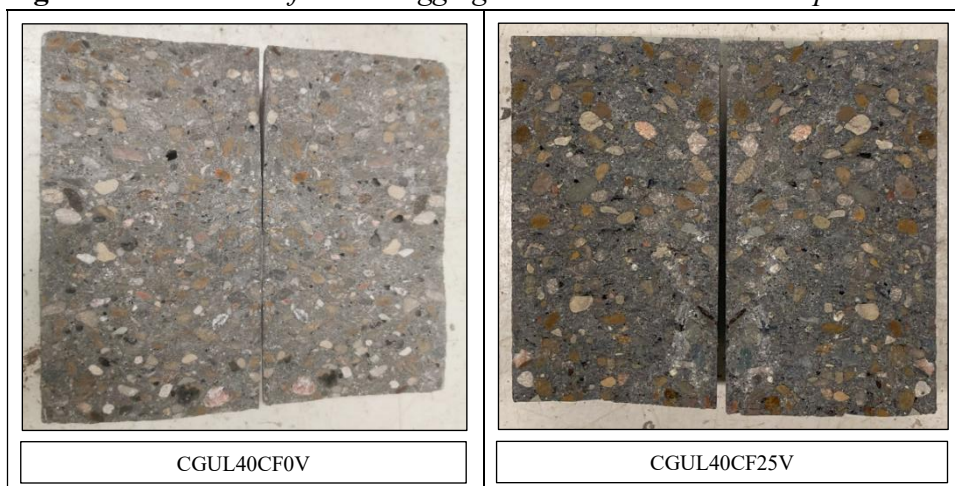
Figure 9. Distribution of Coarse Aggregates in Hardened SCCs Prepared with VMA
