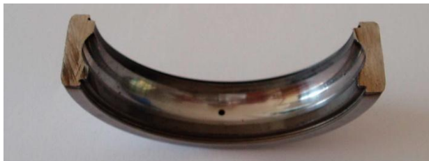
Figure 4. Damage to the Outer Ring of Ball Bearing
