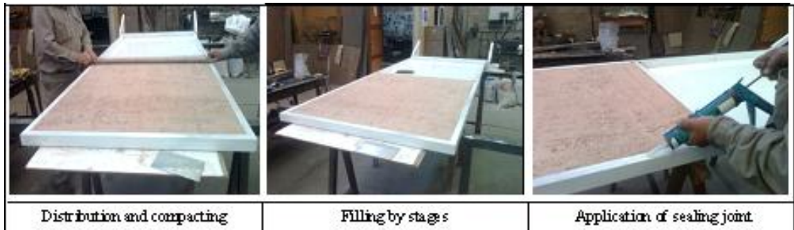
Figure 6. Process of Filling and Finishing for the Final Assembly with Unsifted PP
