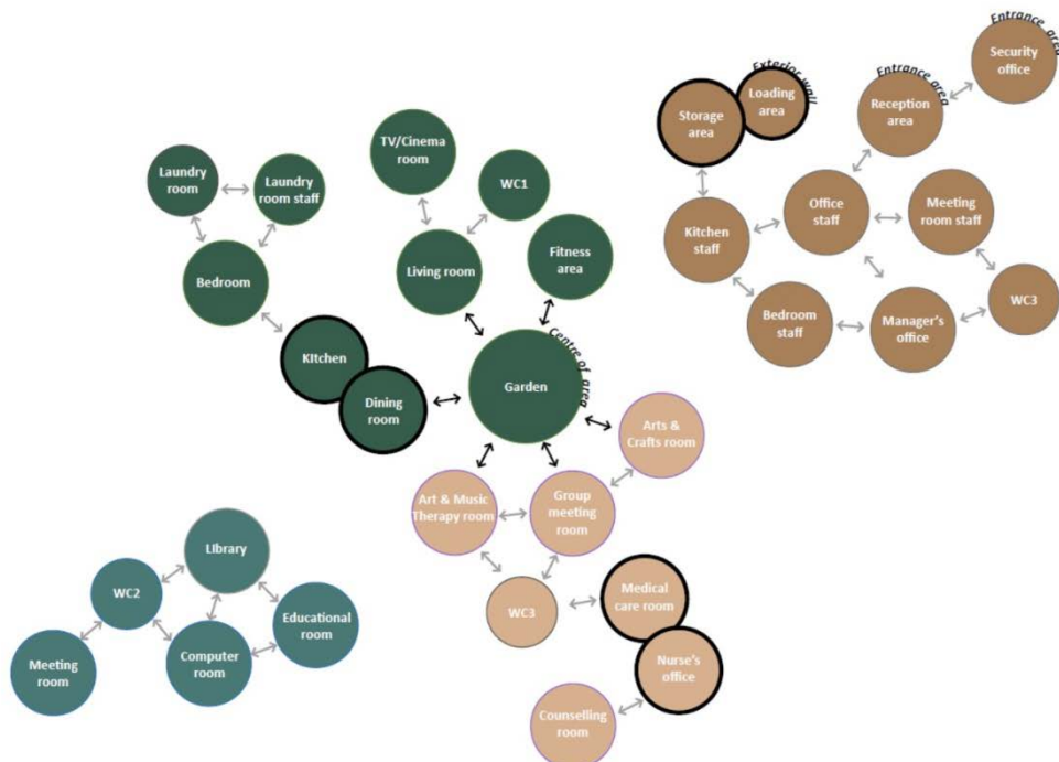
Figure 4. The Network of Adjacencies of Spaces. Activities are Here Represented as Nodes in a Graph Structure. Different Colours Indicate Different Clusters of Activities, Following the Adjacency Study
