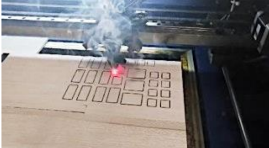
Figure 25. Laser Cutter Process
