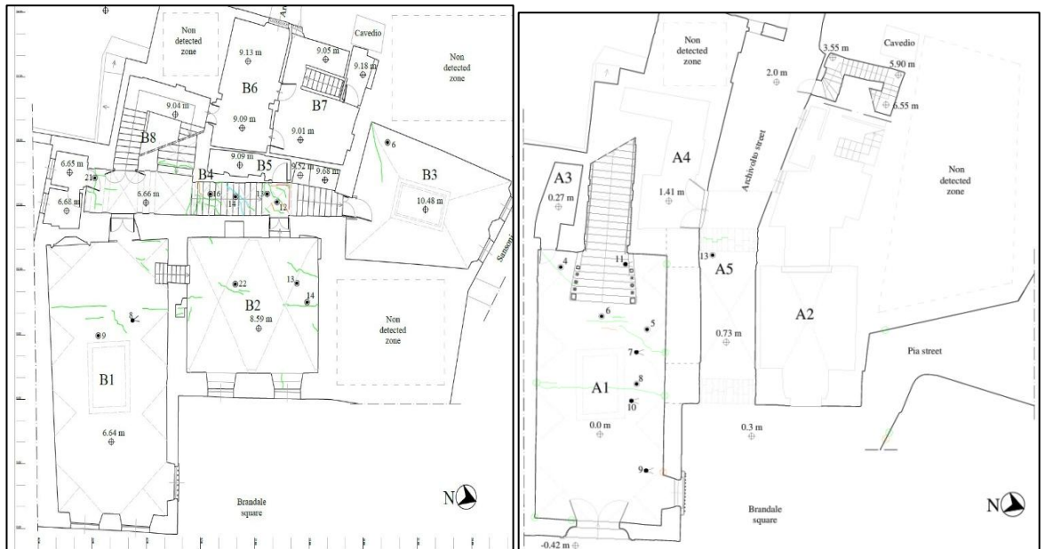
Figure 3. Plan of the Ground Floor – Crack Pattern of Vertical Elements.
