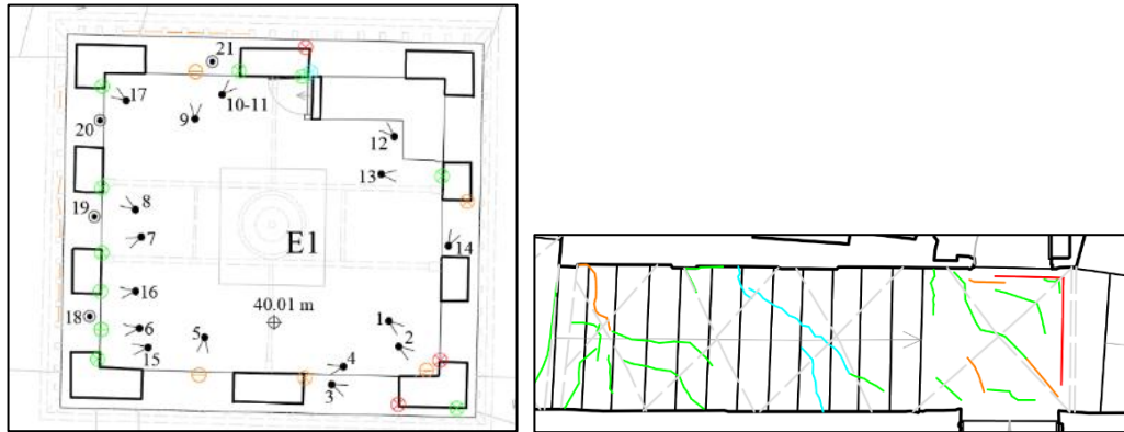
Figure 10. Plan of the First Floor - Crack Pattern of the Vault in Space B4.
