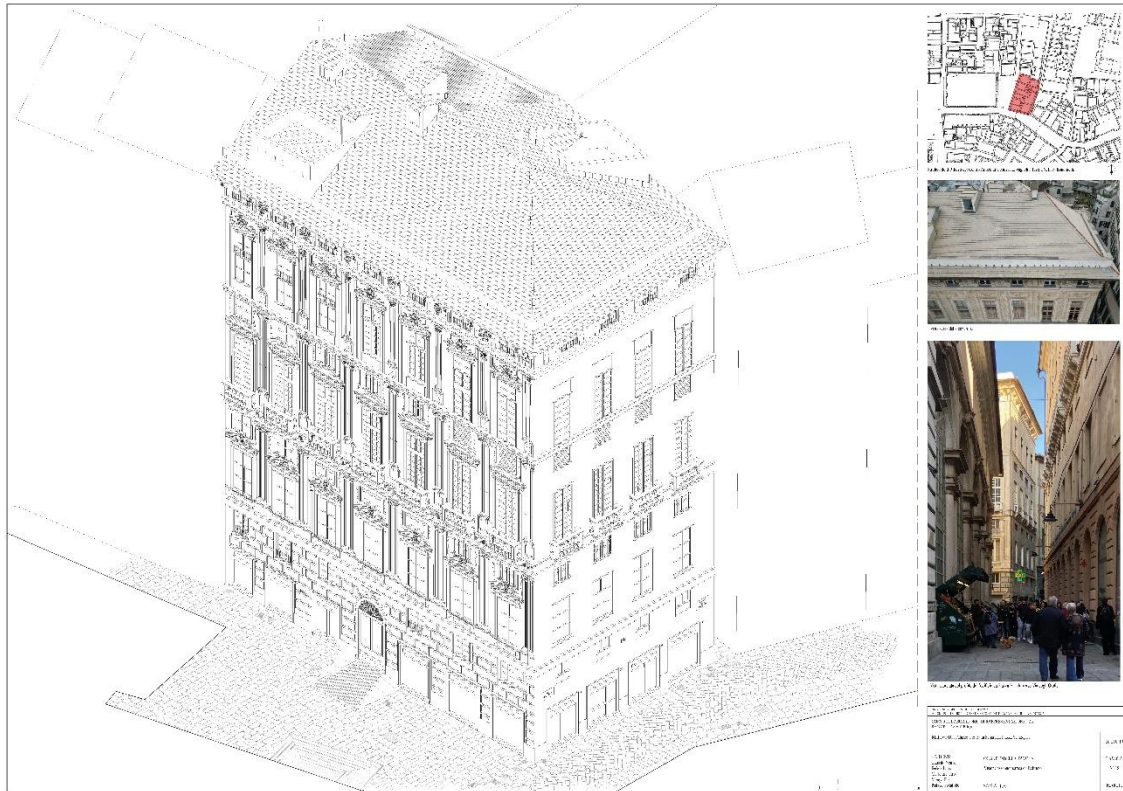
Figure 8. Three-dimensional Reconstruction of the Building Overlooking Piazza Senarega (Genoa), obtained by means of an integrated Digital Survey and Subsequent Interpretative Restitution
