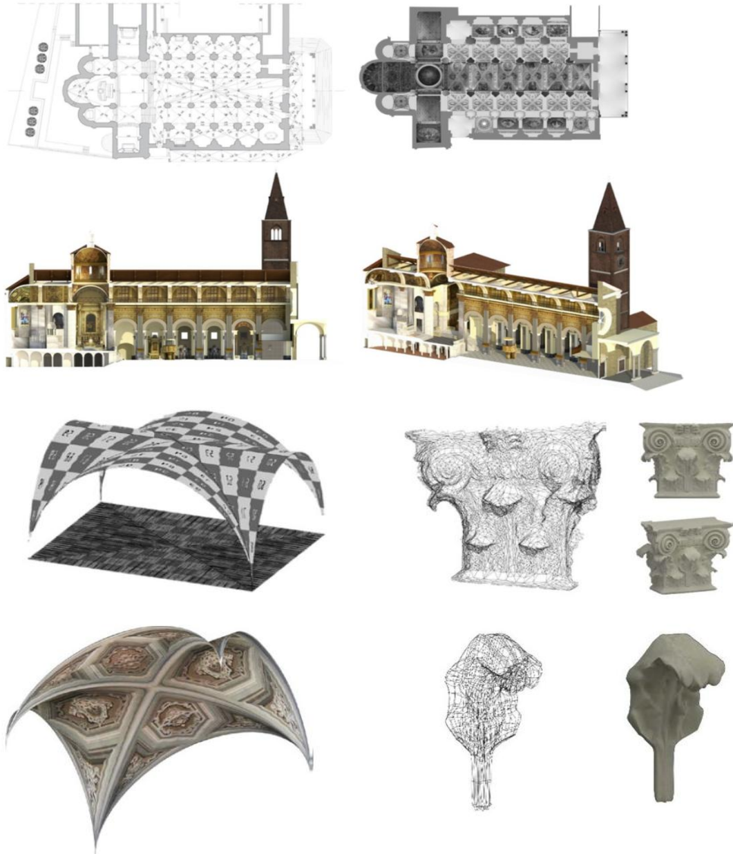
Figure 6. Comparison of a Dimensioned Plan obtained by Direct Survey (trilateration) and Hyposcopic Plan obtained by Digital Photo-straightening Techniques; Rendered Longitudinal Section and Rendered Longitudinal Cutaway; Three-dimensional Modeling of a Vault of the Side Aisles taking up the Concepts of descriptive geometry projected on the Plane for the Mapping; Digital Model of the Capital via sfm and Render
