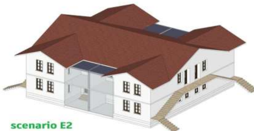
Figure 10. BIM Model Comparing Scenarios for Different Energy Contributions in the Integration of Greenhouses in Building Type “1A” in Panzano District: From Top to Bottom, State of Fact, Greenhouse Integration, Greenhouse Integration with Solar Photo-voltaic Integration on Rooftop Source: Authors 2025.
