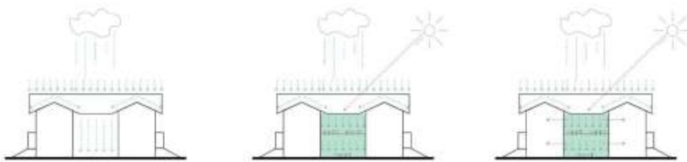
Figure 12. Comparative Diagram for Assessing the Potential Contribution of the Bioclimatic Greenhouse and the Integrated System in Supporting Three Forms of Self-sufficiency: i) Water, through Rainwater Harvesting and Reuse; ii) Energy, through the Reduction of Energy Demand for Heating and Cooling; Food, by Enabling Small-Scale Domestic Vegetable Production
