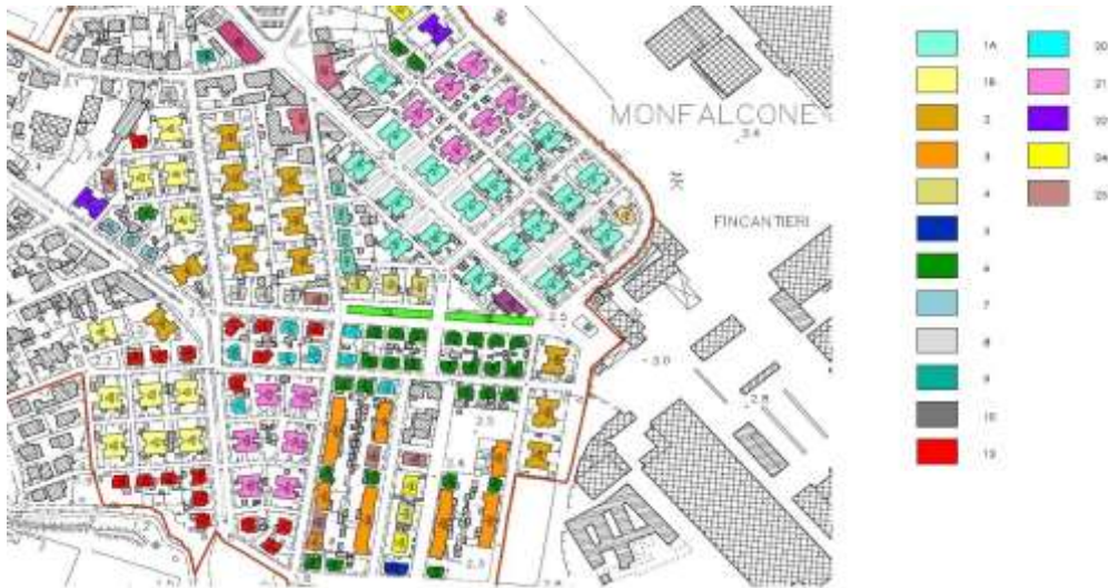
Figure 6. Situation Plan (2010) of the Building Stock Typologies in the Workers' Village: The Continuous Red Line Borders the Perimeter of the Recovery Plan Scope. In the Key Legend, Codes 1A and 1B Refer to Eight-dwelling Houses with Separate Entrance, which Constitute the Focus of this Study
