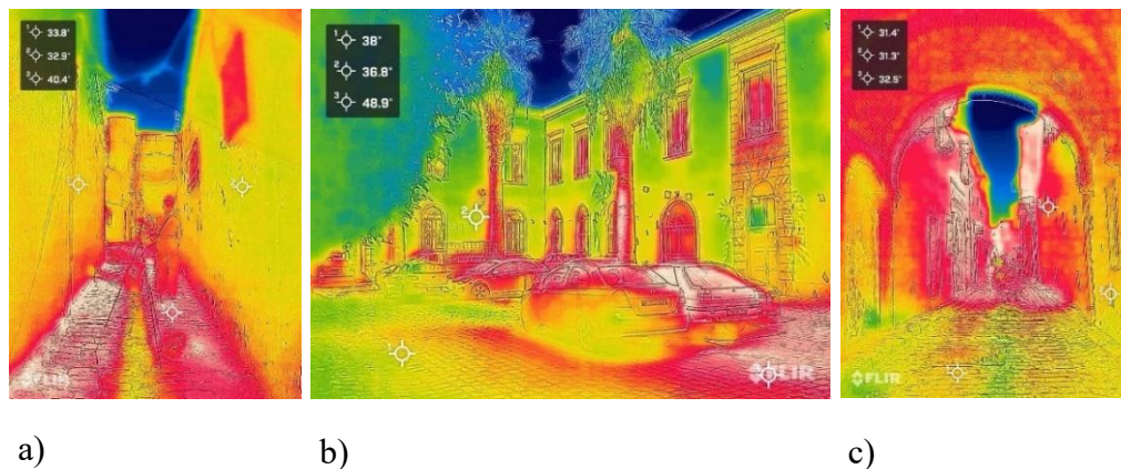
Figure 8. Representative Thermal Images Captured during the Afternoon Measurement Period (14:00–15:00) Showing Surface Temperature Distributions in the Three Urban Typologies: (a) Alley: Rue La Noria (P1), (b) Placette: Palais Kheireddine (P2), and (c) Sabbat: Rue du Pasha (P3)
