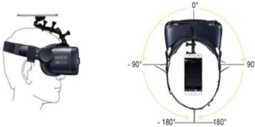
Figure 4. Experimental Setup: VR Glasses with Coupled smartphone and Attitude-sensors
