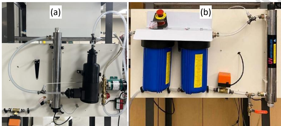
10 11 Figure 3. Water Filtration System Developed by SEPT Learning Factory
