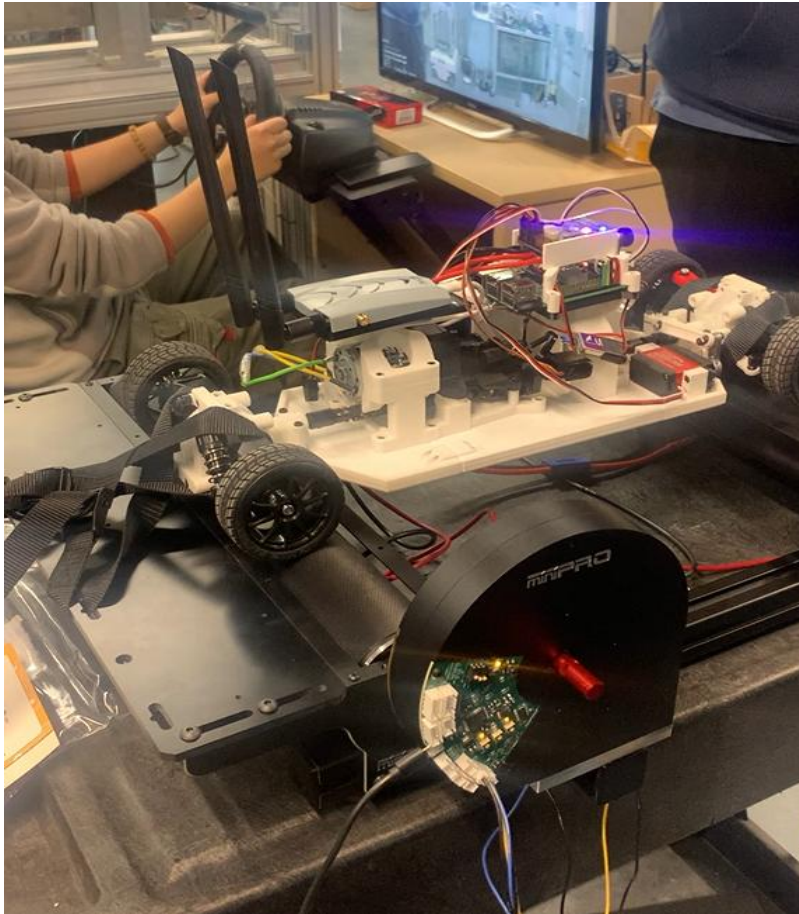
1 Figure 1. Testing Performance of RC Car on Dyno at SEPT Learning Factory
