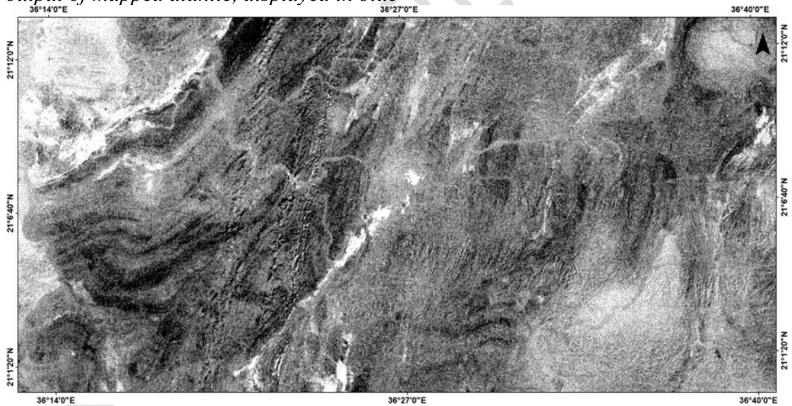
Figure 12. Alunite Index derived from ASTER data: (a) band ratio image ((Band 7 / Band 5) \times (Band 7 / Band 8)), highlighting alunite-rich zones; (b) vectorized output of mapped alunite, displayed in blue
