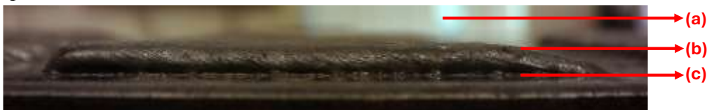
Figure 1. Raw side-profile photograph of a steel WAAM bead on substrate plate
