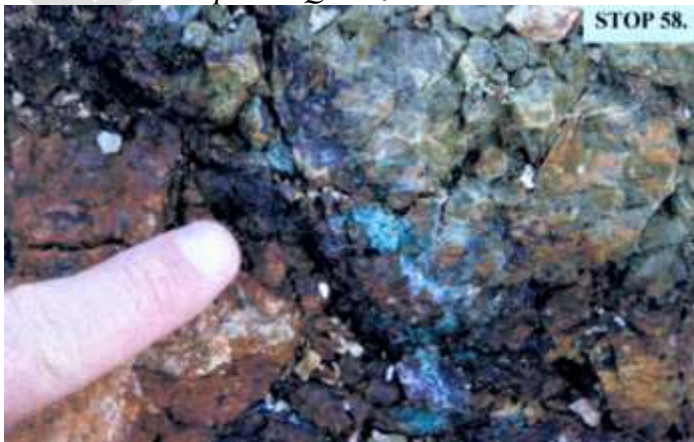
Figure 27. Copper Minerals: Chalcopyrite, Bornite, Pyrite and Malachite and Limonite in the Epidote-Quartz Veins
