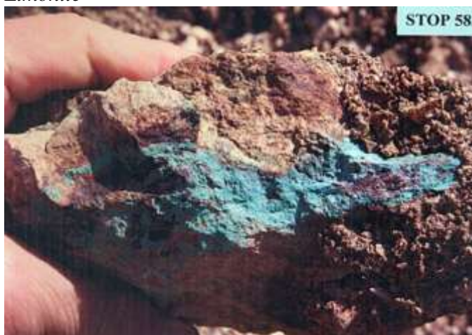
Figure 28. Copper Mineralization - Highly Weathered Rock, with Malachite and Limonite
