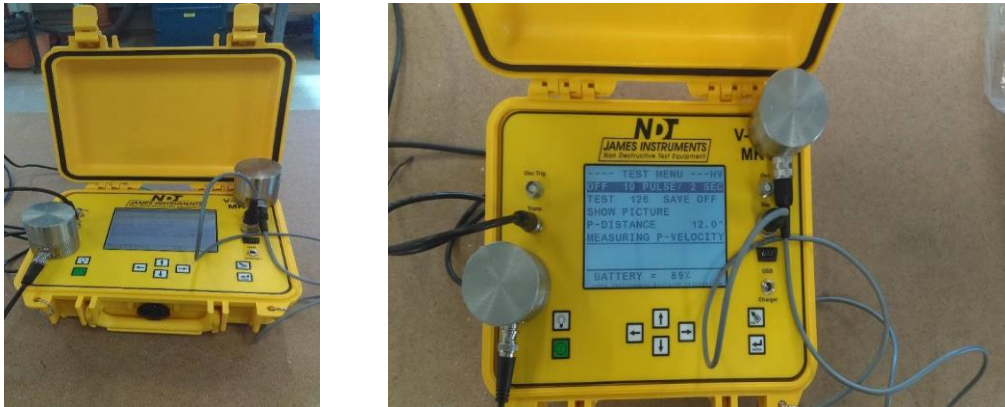
Figure 3. Ultrasonic Pulse Velocity Equipment
