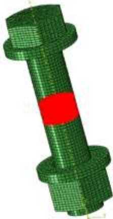
Figure 8. Mesh and Load of the Bolt
