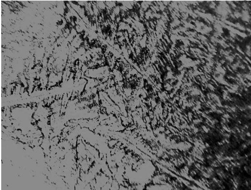
Figure 3. b) Austenite SS Cladding, 200X, Etchant: Ralf's Reagent
