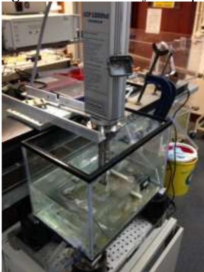
The under-investigation specimens, shaped in small rectangular plates, were mounted onto the base plate, positioned at the bottom of tank, which was then filled with fresh water. The head of the ultrasonic transducer (sonotrode) was placed just above each specimen's surface at a predetermined distance of 1mm. The base plate, as well as each specimen, had got markings to ensure correct placement, every time a specimen was taken out for measurements.
