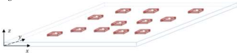
Figure 7. Non-Collocated Piezoelectric Patches Bonded on a Plate
