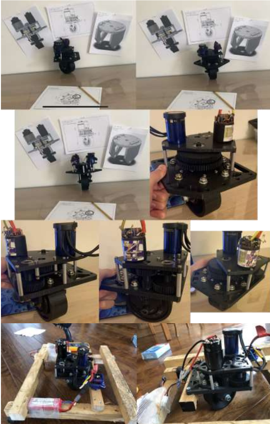
Figure 11. Several Images of the Prototype Swerve Drive Module, Along with the Images of the Dolly Swerve Drive Prototype Assembly
