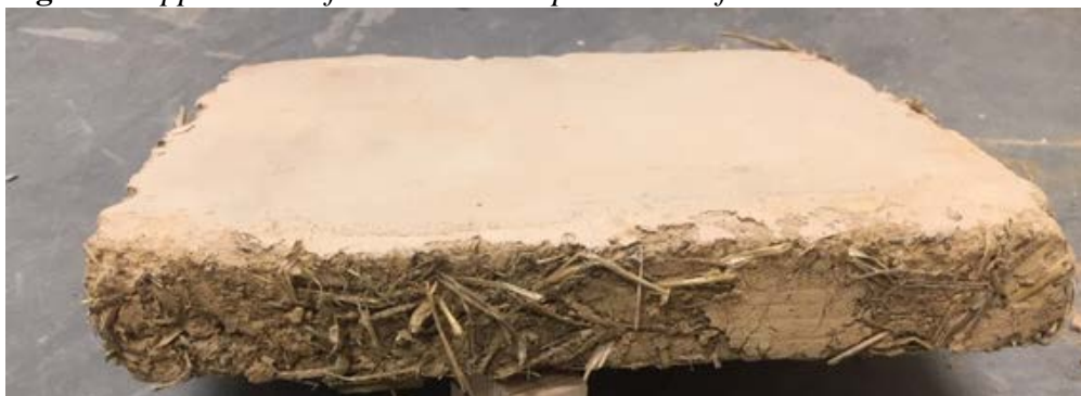
Figure 4. Appearance of the Hardened Specimen Surface
