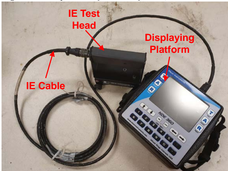
Figure 5. Components of the IE Test Head (Transducer and Solenoid Impactor)
