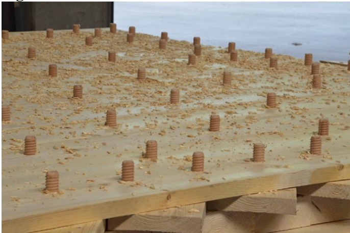
Figure 2. Dowel Laminated Timber Panels
