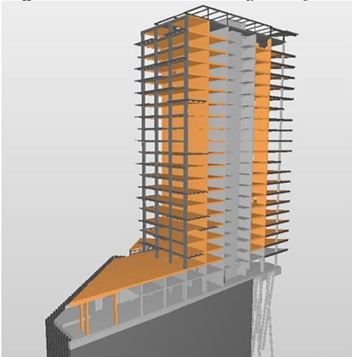
Figure 11. An Isometric Diagram of HAUT Structural System
