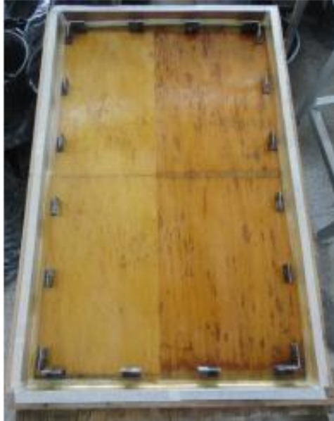
Figure 2. Wooden Molds with Steel Angles
