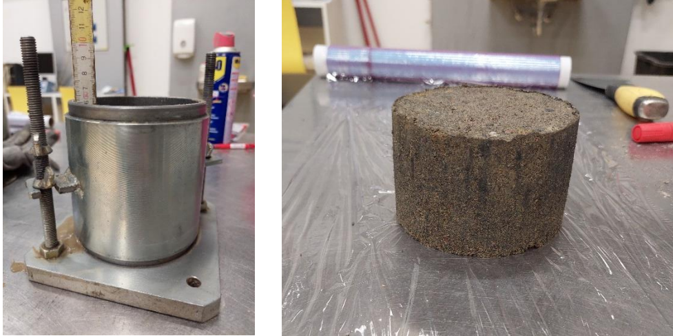
Figure 3. Specimen Production for Cyclic Testing
