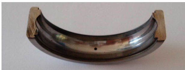
Figure 4. Damage to the Outer Ring of Ball Bearing
